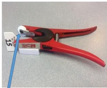
Align the arrow on back side of the RFID and the bump on the front side of the RFID to the front of the tagger.
