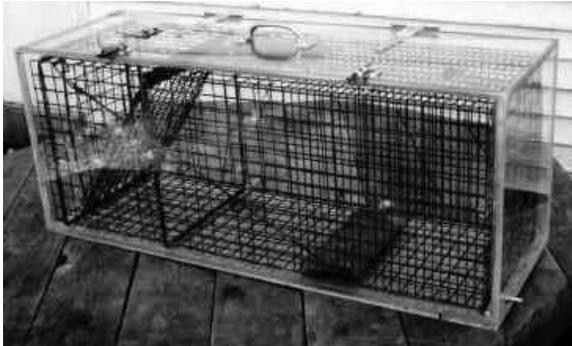
**Figure 1.** A cage trap enclosed in a carbon-dioxide euthanasia chamber constructed with Plexiglas®. Photo by Stephen M. Vantassel.
