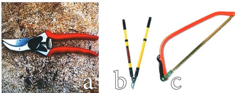
Figure 3. Examples of hand pruning equipment: (a) scissors-cut hand shears, (b) lopping shears, and (c) curved pruning saw. Photos: Oregon State University.
