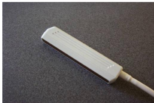
**Picture 1:** An ultrasound transducer houses tiny crystals that emit and catch the sound waves.
