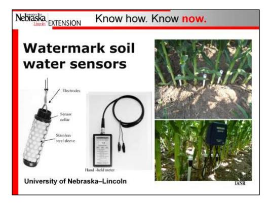
Watermark sensors are used to measure soil moisture to determine irrigation timing and amount
