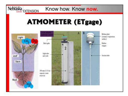
In order to measure a crop's ET, an **atmometer** or **ETgage** can be used.
