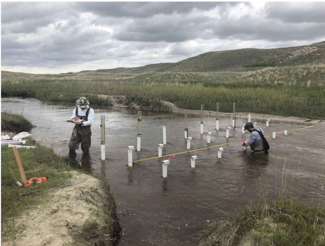
Sampling and measuring groundwater seepage into the South Branch of the Middle Loup River on Gudmundsen Sandhills Laboratory in May 2019. Image courtesy of Mikaela Cherry.
